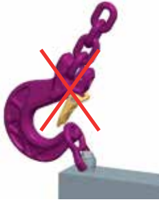
Pic. 5: Only use suitable lifting means for attaching to the ACP.
