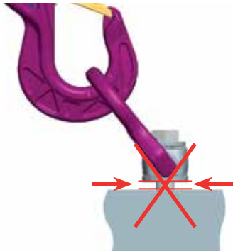
Pic. 7: The lifting point must be fully screwed in.
