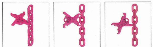
Pic. 27: Patented ICE-lashing chain inspection gauge for an easy inspection of c) and d)
