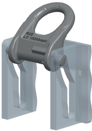
Fig. 3: Permitted assembly alignment (RUD and LC lettering face away from the load)
