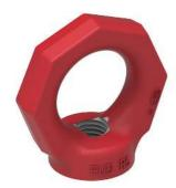
For the RUD RM - eye nuts, the threaded connector component must be of atleast quality grade 8.8
