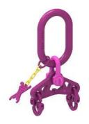
ICE - Master link for assemblies with ICE - balancers. When using two units of 2 leg slings, where by one of which is equipped with a balancer (IWK-2S-10) and both master links are in the crane hook, the calculation of the capacity can be based on 4 bearing slings (BGR 500/DGUV Regel 100-500) provided the load is symmetrical and the inclination angle is max 45°. Hence an increment of the WLL. Suitable for crane hooks up to no. 10 acc. to DIN 15401
