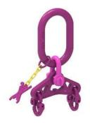
ICE - Master link with B=190 mm for assemblies with ICE - balancers. When using two units of 2 leg slings, where by one of which is equipped with a balancer (IWSAK 2S) and both master links are in the crane hook, the calculation of the capacity can be based on 4 bearing slings (BGR 500/DGUV-Regel 100-500) provided the load is symmetrical and the **inclination angle is max 45°**. Hence an increment of the WLL.
