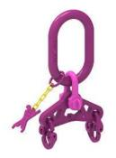
ICE - Master link with B=250 mm for assemblies with ICE - balancers. When using two units of 2 leg slings, where by one of which is equipped with a balancer (IWSAK 2S) and both master links are in the crane hook, the calculation of the capacity can be based on 4 bearing slings (BGR 500/DGUV-Regel 100-500) provided the load is symmetrical and the **inclination angle is max 45°**. Hence an increment of the WLL.
