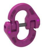
The all-purpose ICE - coupling link. The connecting pin is held by a reliable safety tensioning sleeve. It does not move around and hence less vulnerable to being damaged. On to the link brackets, various extrinsic connections eg: lifting points, grabs and chains can be mounted.
