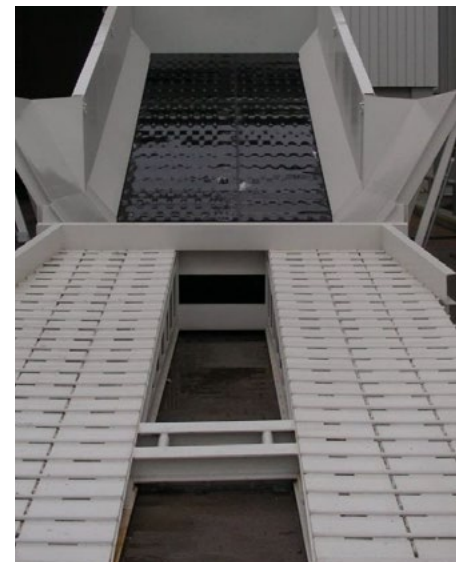
RUD unloading ramp system for truck unloading into the conveyor.
