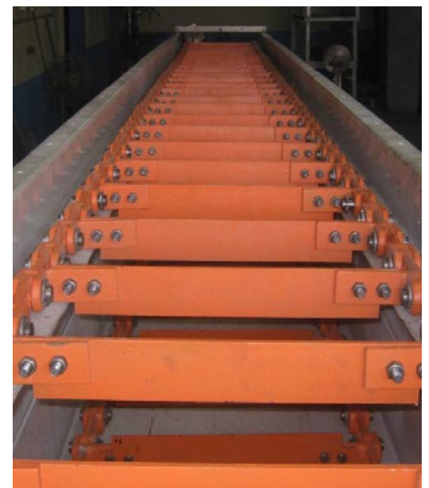
Drag chain systems remove dust, and collect the product for further processing or storage.
