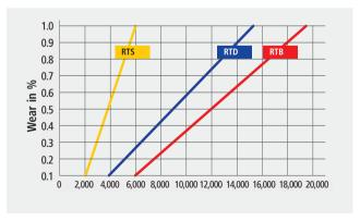
The quality classes relate to material, chain design and production process. Values given in case of test stand testing. Drive wheel, chain guide and scraper all designed and fabricated to to the state of the art.
