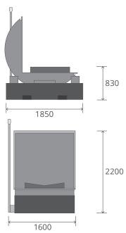
Weight: 1600 kg Working Load Limit (WLL): 6000 kg
