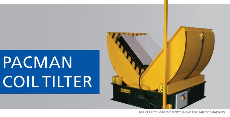
The Pacman Coil Tilter is a small footprint upender for tilting coils of steel from a vertical to a horizontal bore position enabling safe loading to an Uncoiler machine. It is mechanically driven and can be stopped with the load held at any point in the turning process. This machine is robust, easily maintained and reliable with quality Australian-sourced componentry. Our 6 tonne model is standard and we can also manufacture to suit the tonnage required.
