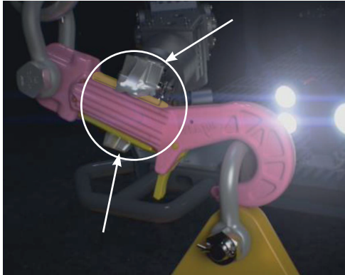
Fig. 6: Press the release/locking and the securing latch
